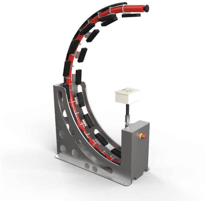
**System for 360° testing in one shot for mono block tubes**
