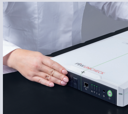
Daily check of the collimator size indicator
