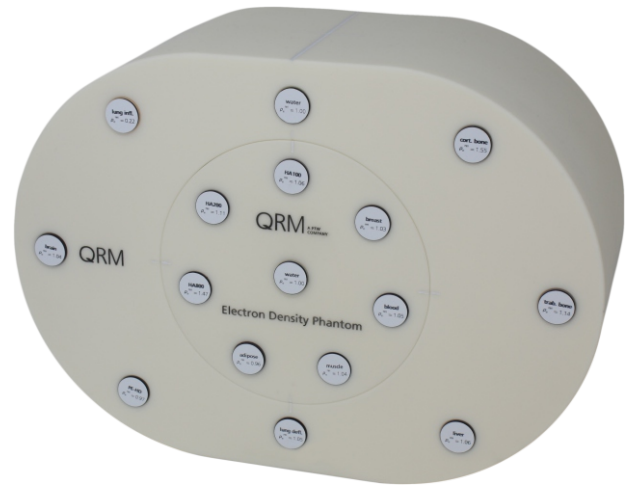
Comprehensive Electron Density Phantom (QRM-C-EDP)
