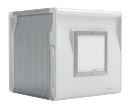
**QUBENEXT** is an MLIC-detector for the measurement of depth dose curves. The base version contains 4 modules allowing a measuring depth of 77 mm wet (2.4 mm resolution). The sensitive area is 127 mm x 127 mm. Additional modules for a wet of about 300 mm max and an xy-detector-add-on are available.
