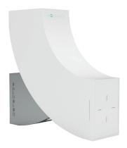
**AQURACY** is a detector to measure radiation characteristics in a single beam shot. The data comes from a 50 mm diameter scintillating screen and CCD camera. The resolution is 10  $\mu$ m.
