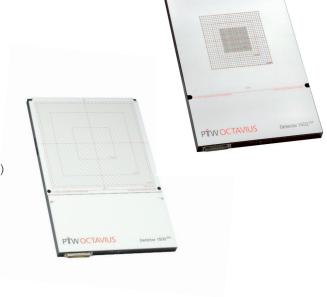
(1500 XDR) and 2.5 mm x 2.5 mm x 2 mm (1600 XDR) in size. The square chamber design of the OCTAVIUS Detector 1500 XDR offers 50 % field coverage and the design of the OCTAVIUS Detector 1600 XDR offers unique 100 % field coverage in the central region. Read out cycles of 100 ms provide the basis for real-time analysis of beam profiles.
