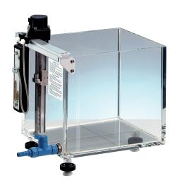
**MP1 1D Water Phantoms** (T41019/T41025) for reference dosimetry and measurement of depth dose curves, motorized or manual
