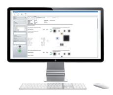
PQASoft is a software to check the consistent performance of pencil beam scanning systems in particle therapy. It has been designed for easy e.g. daily checks of beam properties, i.e. beam positioning, spot size and shape, field flatness and energy constancy.
